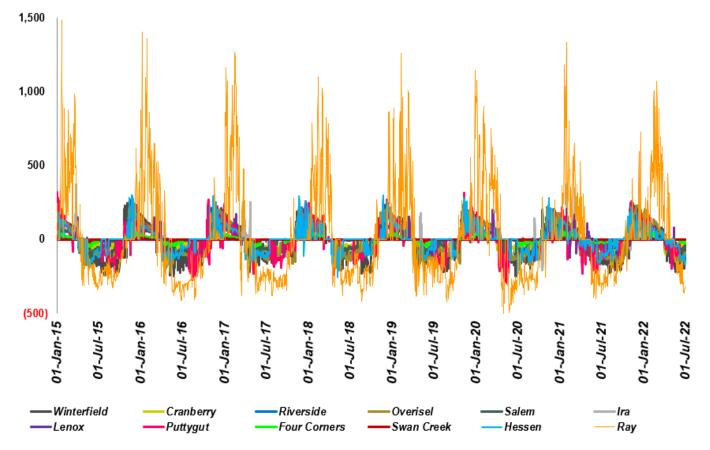
Figure 16: Daily Storage Field Injections (negative) and Withdrawals (positive) by Field from January 2015 - July 2022 (mmcf)
