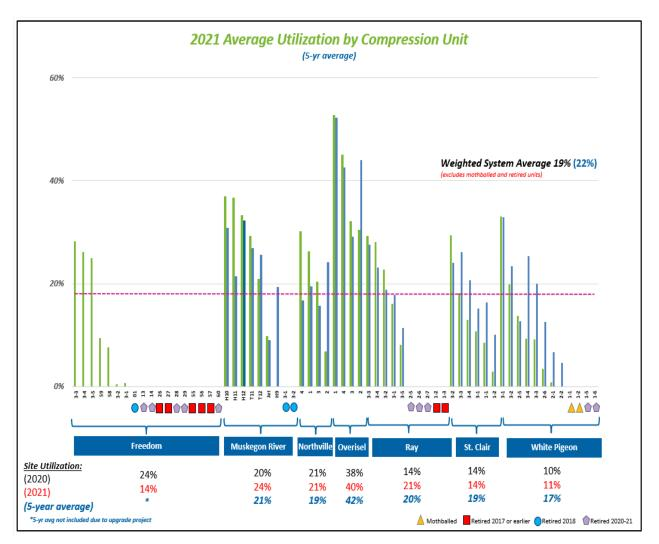
Figure 21: 2021 Average Utilization by Compressor Unit
