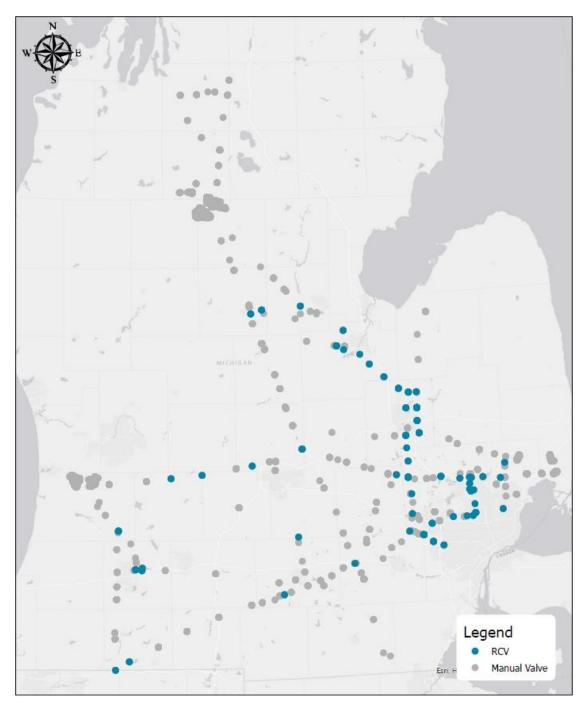
To leverage RCVs as a means of increasing the safety of the transmission system, the Company is planning an installation rate toward a goal of 70% of the system valves by 2028, as shown in Figure 32.
